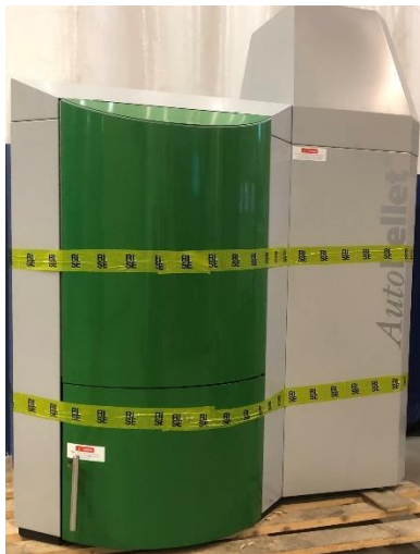
Figure 1b Sealed boiler after testing
