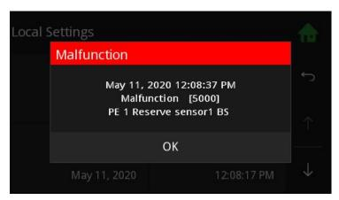
Fault messages can overlayed on all menu items and appear immediately if a fault occurs. Every fault message appears with the date, time and name on the display. It remains until it is acknowledged.
