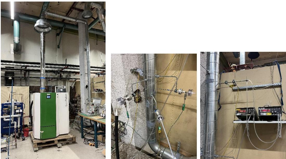
Figure 1b. boiler in test rig and measurement installation and setup
