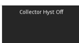
If the temperature difference between the collector sensor and TPU, ACC lower sensor is lower than the Coll Hyst A, the solar pump switches Off.
