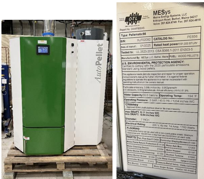
Figure 1d Resealed boiler after testing at RISE
